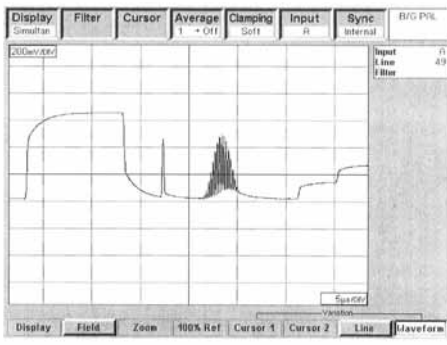
Fig. 2.20. Linearly distorted white pulse, 2T pulse and 20T pulse
